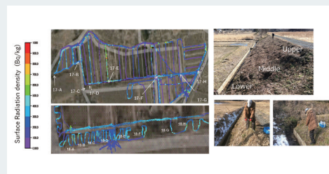
放射性セシウムの表面汚染密度校正(福島県飯舘村) Surface contamination density measurement of radioactive cesium (Iitate village, Fukushima)
